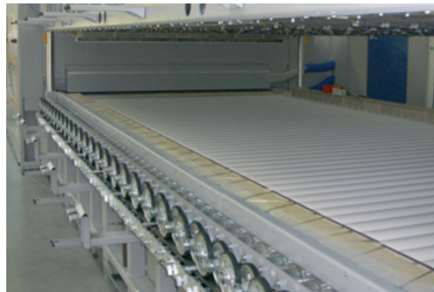
Glass tempering furnace with HalRoller-FS
