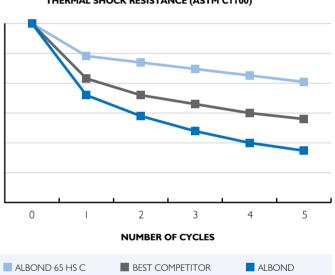
THERMAL SHOCK RESISTANCE (ASTM CI100)
